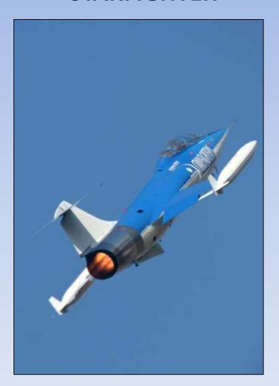
The Lockheed F-104 Starfighter is the highest performance, single-engine jet fighter ever made. The F-104 is powered by a single General Electric J79-GE-11A engine capable of generating in excess of 17,000 lbs of thrust and exceeding Mach 2. For perspective, that's roughly equivalent to 36,000 horsepower, or more than the entire starting line-up at the Daytona 500.
